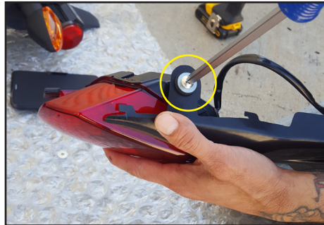
14) Use stock hardware to mount tail light to undertail.
