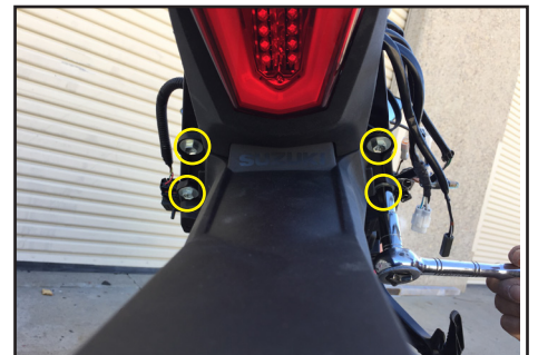
9) Remove 4 bolts holding under tray.
