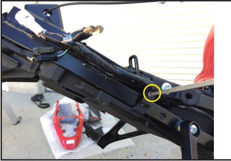
10) Remove side screws holding under tray.
