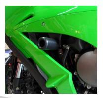
Hotbodies Racing frame sliders serve the purpose of mitigating damage to the motorcycle. Although statistics have shown that frame sliders reduce damages to the frame, cases, swing arm, and levers there is no guarantee that this product will eliminate damage all together in the event of a crash.
