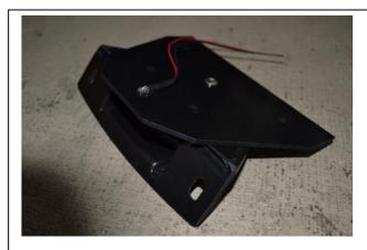
6) Line up the mounting plate w/LED license plate light over the tag bracket and secure snugly with the phillips screw provided.
