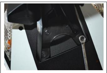
1) Remove stock fender bracket by first removing the 4 10mm bolts under the tail section.
