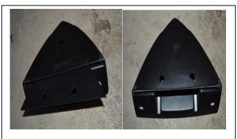
5) Prepare the new tag bracket for installation. Insert flat piece w/3 holes into the main tag bracket. Use Rubber well nut to hold pieces together.
