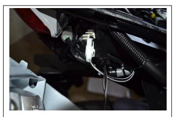
4) Locate white license plate light plug on the inside of the tail piece and unplug. Feed plug through hole in undertail and remove the stock fender.
