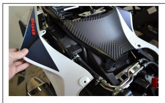
3) Remove 4 pop rivets on right side of tail located around the trunk compartment, underneath right side of tail section, and also the one phillips screw by the rider seat.
