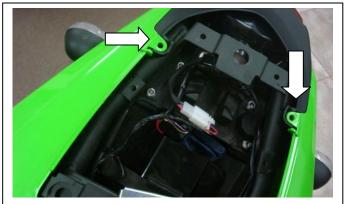
1. Remove the rear seat, and bolts securing the tail fairing.
