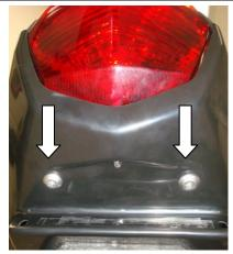
9. Slide the Hotbodies Racing Tag bracket around taillight. Fasten through both of the brackets and the sub frame with stock bolts, and supplied nuts.
