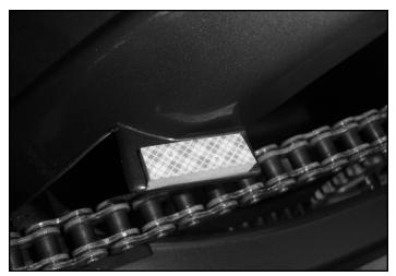
2) Use stock pop rivets and screws to re-install hugger. Use provided double-sided tape to connect the hugger to the chain guard. If not installing a chain guard, you may remove the tape.
