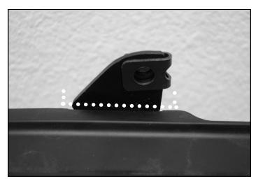
**2)** Remove the plastic shown in the photo above if you do not want to see this piece exposed after the installation.
