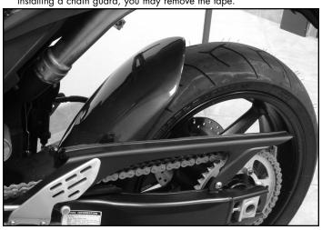
**3)** Tighten all hardware on hugger and chain guard, using all stock mounting hardware. Your done!
