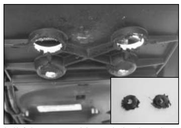
2) Using a "Dremel" tool or cutting disc (this can also be done using a sharp edged knife, but is not recommended), remove the plastic shown in the photos above and below. Be sure to take your time cutting, so that you don't cut away any more plastic than necessary.
