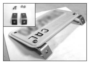
3) \*Install license plate brackets to back side of license plate as shown. Now hold license plate in desired location on undertail (under the signals), carefully mark and drill holes, install using the two (2) sets of bolts & nuts.
