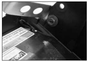
3) Now relocate the rear mounting holes for the glove box 1.25" lower in the tray to raise it up in the subframe as shown.
