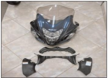
1) Remove entire front upper fairing. Including headlight, mirrors, windscreen, and dashboard pieces for easier installation of air scoops.
