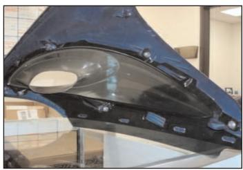
**4)** Once stock cover and turn signal is removed, install Hotbodies air scoops. Re-use phillip head bolts to secure scoops to upper fairing.
