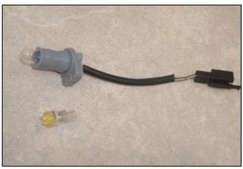
**5b)** To install signals in headlight, remove running light plugs from headlight housing. as pointed out in photo 5a. Replace stock bulb with provided amber LED marker, plug running light back in to headlight housing and re-wire.
