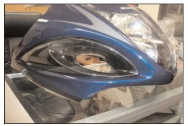
**6)** Once headlight is securely installed, re-install upper fairing with all appropriate hardware, including mirrors, windscreen, and covers. Re-connect all wires, and wiring harness, making sure everything is in place and secure. Your Done!
