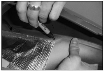
2) When tail section body work is removed, line up the undertail with tail section carefully marking holes from bottom to top, respectively on each side. Make sure tail is correctly lined up with tail section.
