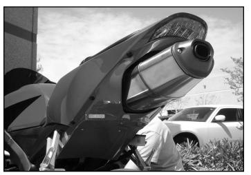
5) Make sure your exhaust is fully tightened and re-install all tail section plastics and connect the LED turn signals to the undertail. Use the plastic screw rivets to connect the undertail to the tail section.
