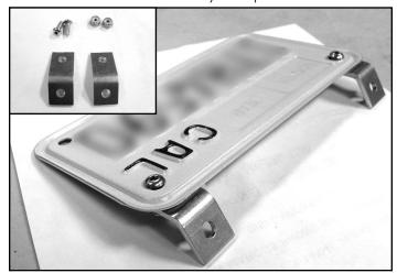
4) Install license plate brackets to back side of license plate as shown. Now hold license plate in desired location on undertail where it will not hit the rear tire. Carefully mark and drill holes, install using the two (2) sets of allen bolts and lock.
