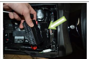
7) Re-lease the latch on the fuse box then lift up and move to the side. Remove the small phillips head bolt located behind the box.
