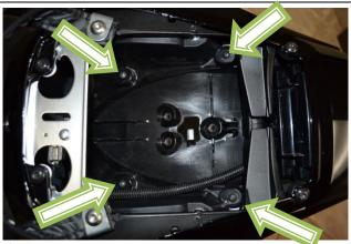
8) Remove the 4 remaining phillips head bolts located inside the glove box and carefully remove the stock undertail.
