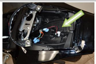
12-A) Picture shows license plate wires feeding through the hole in middle of glove box.
