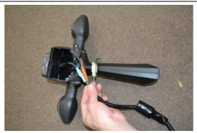
6) Cut the wires closest to the signal lights and remove wiring harness from mudflap. This will allow you to re-use your stock plugs when you hooking it up to the new undertail.
