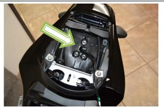
3) Using a 10mm socket and ratchet, remove the 3 bolts located directly below the passenger seat holding the mud flap on and carefully remove it.
