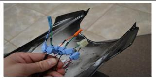
11) Prepare HBR undertail for installation. Connect your factory wiring harness to the undertail. Use wiring instructions down below. Note (you can also drill out your undertail for the license plate at this time, but be sure to check the position for clearance with the rear tire with suspension travel.) 12) Carefully feed signal wires through tail section and license plate wires must be fed through the hole in the stock glove box so that they do not get in the way of the new undertail. (12-A)
