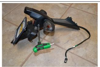
4) Remove the two 5mm hex head bolts on the sides of the mudflap.
