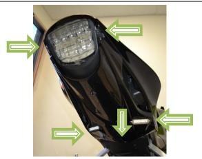
12-B) Pictures shows undertail in position for final installation, arrows mark mounting tabs and fastener.
