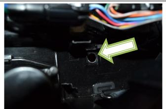
9) Use an electric drill and 3/8" bit to open up that hole that is located behind that fuse box in step 7.
