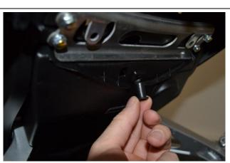
10) Insert rubber well nut from bottom up through the battery box, so the fat part is underneath the tail.
