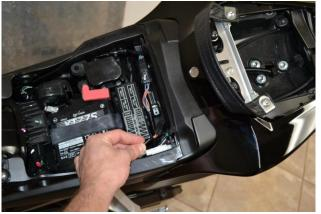
2) Follow the wires from the mudflap back towards the battery box and disconnect the plug from the harness.
