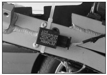
3) Install relay on subframe using zip-tie. (not provided)
