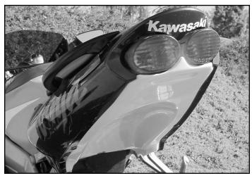
**5)** Re-install all body work leaving all fasteners loose. Now insert undertail into place, right side first, then left, then using stock "pop rivets" insert into body work and undertail tighten, adjust undertail if necessary and re-tighten all stock fasteners, your done.
