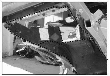
2) Using a "Dremel" tool or cutting disc remove the plastic shown in the photos to the above. Be sure to take your time cutting, so that you don't cut away any more plastic than necessary.
