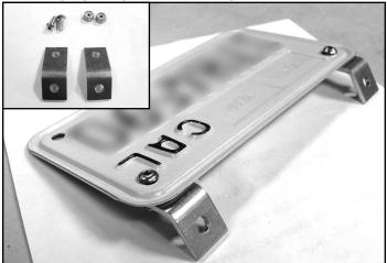
**4)** \*Install license plate brackets to back side of license plate as shown. Now hold license plate in desired location on undertail (under the brake light hole), carefully mark and drill holes, install using the two (2) sets of bolts & nuts.
