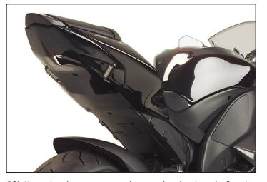
**10)** Align side tail section pieces with new undertail and attach all stock mounting bolts. Re-attach seat and your done!
