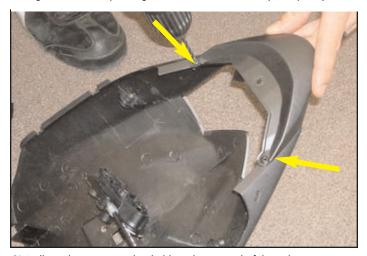
**3)** Drill out the two rivets that hold on the top end of the tail section to remove top piece (as shown in photo). Seperated top end piece will bolt on to new undertail with nuts and bolts supplied.
