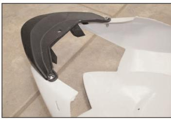
**6)** Attach black plastic piece that was removed in Step 4 and attach to the new undertail with provided nuts and bolts.
