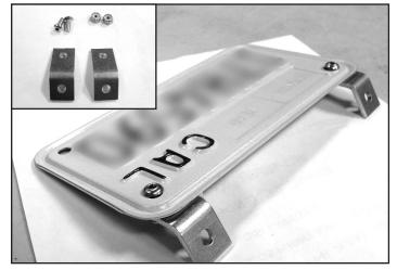
9) \*Install license plate brackets to back side of license plate as shown. Now hold license plate in desired location on undertail, carefully mark and drill holes, install using the two (2) sets of allen bolts and lock nuts.
