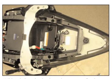
**5)** Slide Hotbodies undertail in place and re-mount using all stock poprivets to attach undertail and sides of fairing as well. Re-mount and connect taillight. Wire in new turn signals and license plate light. \*Wiring directions below.
