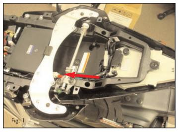
1) Remove stock seats, bolts and pop rivets along the undertail, holding the top tail section to the frame. The top part of the tail can now be removed.
