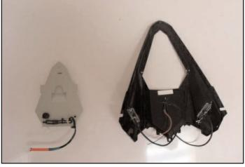
**4)** Disconnect tail light clip and unclip stock undertail. Then remove tail light from stock undertail.
