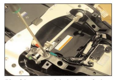
**6)** Re-install aluminum seat mount, latch and crossbar using all stock hardware.
