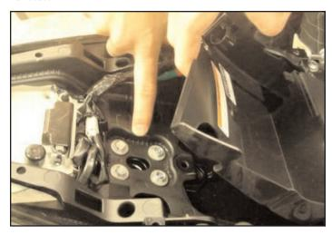
**3)** Lift up on battery box to access 10mm mudflap bolts. Disconnect tail light, signal and license plate light clips. Remove four bolts and detach stock mudflap.
