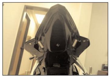
**7)** Re-install stock tail section with all stock bolts and hardware. \*Note tail light will not bolt up to the new undertail, when everything is securely mounted, taillight will be snuggly fitted between new undertail and subframe. Re-install seats and your done!
