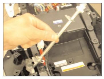
2) Remove two bolts that mount seat latching crossbar to subframe. Move bar and latch off to the side. Remove aluminum bracket as pointed out in Fig. 1. Be sure to save all hardware for reinstallation later.
