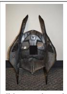
6) Separate the stock undertail from the tail section & the tail light. Be very careful not to break the tabs along the edges of undertail and tail section. Easiest way is to start with the round tabs in the front and then work your way backwards.
