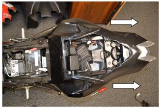
5) The tail section should be loosely mounted on the sub-frame. Slide the entire tail section and undertail assembly backwards and off of the sub-frame.
