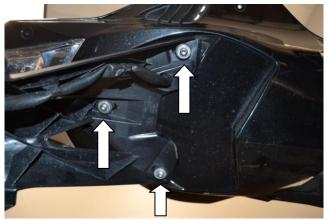
3) Remove the three torx bolts underneath the tail section that hold the mud flap on. Then remove stock mudflap assembly. \*Careful with the wires\*
