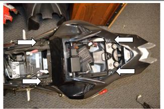
4) Remove the tail section torx bolts located on the top & bottom of tail section, 4 on top & 6 on bottom along the undertail edge.
