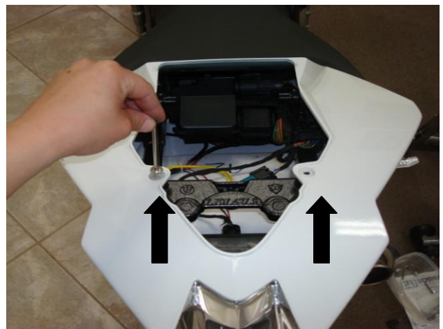
16. Tighten the 2 bolts holding the top tail fairing into place.
