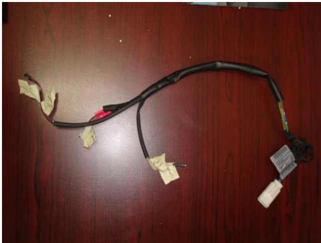
11. Use the stock connector and connect to Hotbodies Racing undertail. (See diagram at end)
