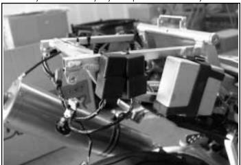
3) Attach the loose relays to the sides of the subframe using 2 zip ties.
