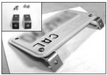
**6)** \*Install license plate brackets to back side of license plate as shown. Now hold license plate in desired location on undertail, carefully mark and drill holes, install using the two (2) sets of allen bolts and lock nuts.
