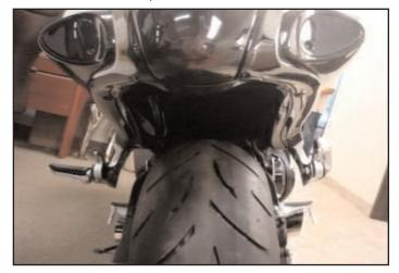
4) Slide new undertail in place and mount with supplied screw rivets.
