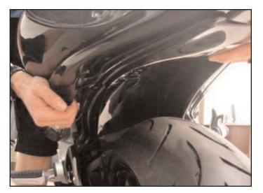
**2)** Remove four pop rivets along tail section including all mounting bolts for tail section. This will allow tail section to move freely, making installation of undertail simple.
