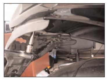
1) Remove solo seat cowl, and unclip license plate wires from harness. Remove 10mm mudflap bolts located underneath tail section. Remove mudflap assmbley and re-install mudflap bolts to secure batterybox.
