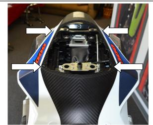
5. Remove the 4 pop rivets that are located on the top of the tail.
