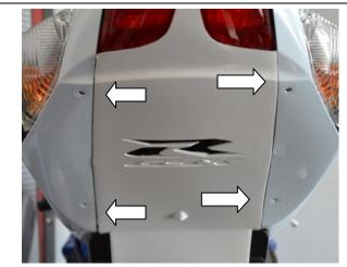
15. Reinstall 4 pop rivets on the bottom of the side tail fairings.
