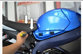
18. Reinstall the front seat, tightening the 2 bolts.
