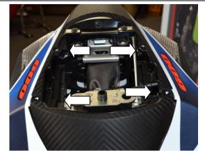
16. Reinstall 4 pop rivets that are located on the top of the tail.
