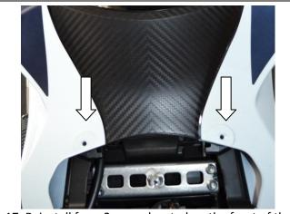
17. Reinstall from 2 screw located on the front of the side tail fairings.
