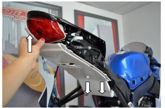
13. Install the new Hotbodies Racing undertail. The tabs at the bottom will be located between the battery box and bolts. The top will clip into place.
