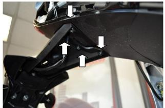
10. Remove the 4 bolts that hold the mud flap to the bike.
