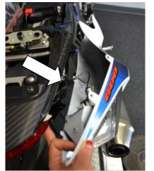
8. Pull right side tail fairing, and disconnect the electrical. Remove from bike completely.
