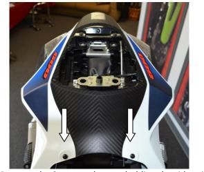
4. Remove the 2 screws that are holding the side tail fairings to the bike.
