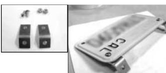
**4)** \*Install license plate brackets to back side of license plate as shown. Now hold license plate in desired location on undertail, carefully mark and drill holes, install using the two (2) sets of allen bolts and lock nuts.
