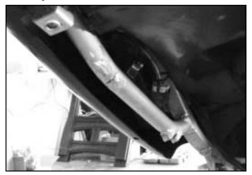
3) Cut cargo net hooks on subframe as shown.
