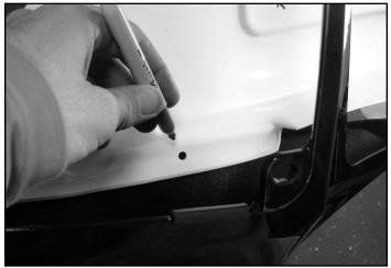
2) When tail section body work is removed, line up the undertail with tail section carefully marking two (2) holes respectively on each side. Make sure tail is correctly lined up with tail section.
