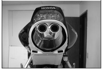
3) After drilling holes, test fit undertail on tail section, checking for proper alignment.
