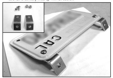
**4)** Install license plate brackets to back side of license plate as shown. Now hold license plate in desired location on undertail, carefully mark and drill holes, install using the two (2) sets of allen bolts and lock.
