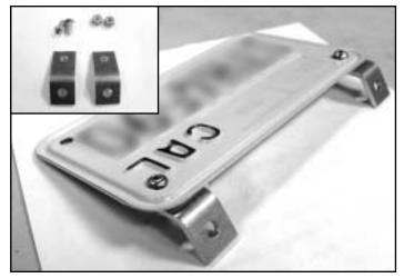
**3)** \*Install license plate brackets to back side of license plate as shown. Now hold license plate in desired location on undertail, carefully mark and drill holes, install using the two (2) sets of allen bolts and lock nuts.
