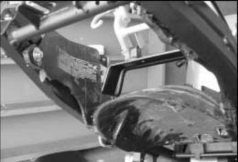
2) Using a "Dremel" tool or cutting disc (this can also be done using a sharp edged knife, but is not recommended), remove the plastic shown in the photos to the above and below. Be sure to take your time cutting, so that you don't cut away any more plastic than necessary.
