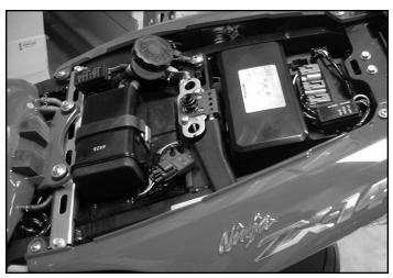
Carefully remove the seat and seat cover, to access trunk compartment of bike. Save all bolts, washers and plastic rivets for re-installation of seat and seat cover.
