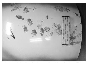
**6)** Before installing the undertail, remove the adhesive back. Carefully clean the stock part where this adhesive will apply to. After you install the undertail with the rivets, press firmly and hold for 30 seconds.
