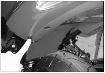
7) Use supplied pop rivets to mount the undertail over top of the stock black trunk compartment and complete wiring of the LED license plate light. To connect the license plate light; use the stock black and yellow tracer wires with black undertail wire and stock red with red undertail wire.
