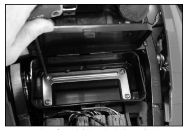
Remove tools and four (4) bolts located at the bottom of tool compartment. Save all bolts for re-installation.
