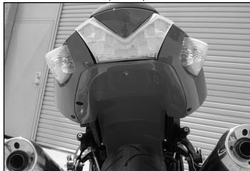
**8)** After mounting undertail, re-install ECU and tool compartments. After re-installation of tool compartment re-install seat and seat cover, making sure all bolts and hardware are fastened securely. Your done!
