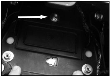
Remove three (3) bolts from mud flap assembly. Stock mud flap should drop down and will be removed.
