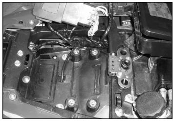
Carefully move tool compartment, ECU and ECU wires out of the way to access mud flap bolts.
