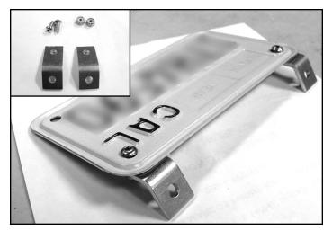
5) \*Install license plate brackets to back side of license plate as shown. Now hold license plate in desired location on undertail, carefully mark and drill holes, install using the two (2) sets of allen bolts and lock nuts.
