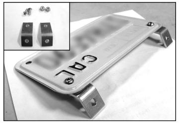
2) \*Install license plate brackets to back side of license plate as shown. Now hold license plate in desired location on undertail (under the signals), carefully mark and drill holes, install using the two (2) sets of bolts & nuts.
