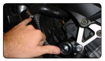
**4.** Install left side offset and frame slider using the longer bolt supplied. Align slider so that it is angled towards the radiator hose fitting. Tighten supplied bolt to manufactures torque specification using a 14mm socket wrench. Tighten slider to the offset using an 8mm allen wrench. Re-install left side mid panel.
