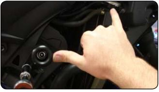
**2.** Install right side offset and frame slider using the shorter bolt supplied. Align slider so that it is angled towards the radiator cap. Tighten supplied bolt to manufactures torque specification using a 14mm socket wrench. Tighten slider to the offset using an 8mm allen wrench. Re-install right side mid panel.
