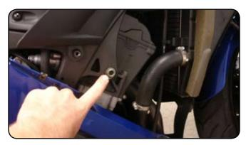
**1.** Identify right slider and aluminum offset. The right slider is the longer slider and is used in conjunction with the longer aluminum offset. Remove right side mid-panel. Remove right side engine mounting bolt. <u>DO NOT REMOVE BOTH</u> ENGINE MOUNTING BOLTS AT SAME TIME!
