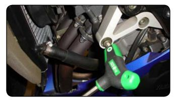
**3.** Remove left side mid-panel. Remove left side engine mounting bolt.
