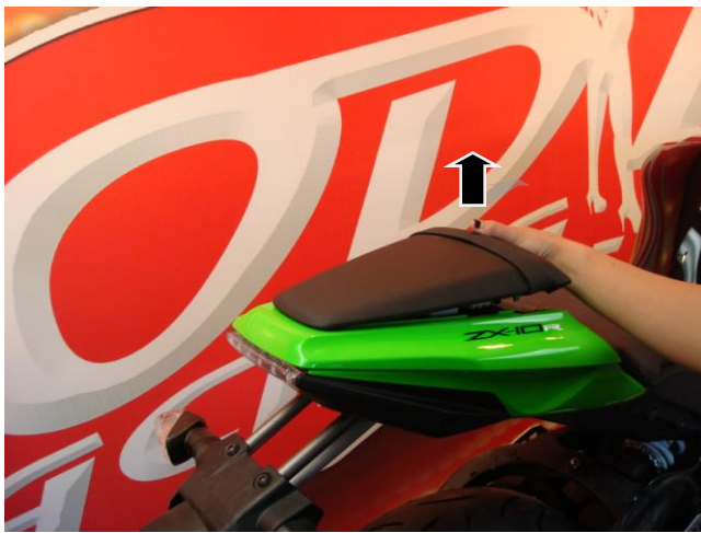
1. Remove the rear seat.
