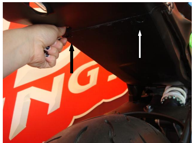
10. Remove bottom pop rivets, and pull undertail to remove.
