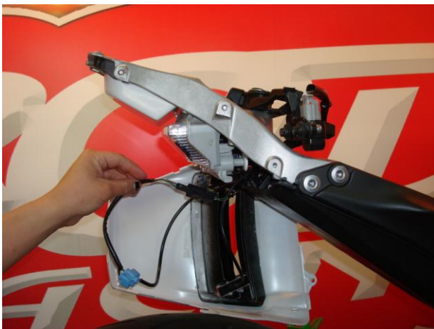
25. Connect the turn signals, and ensure proper function.
