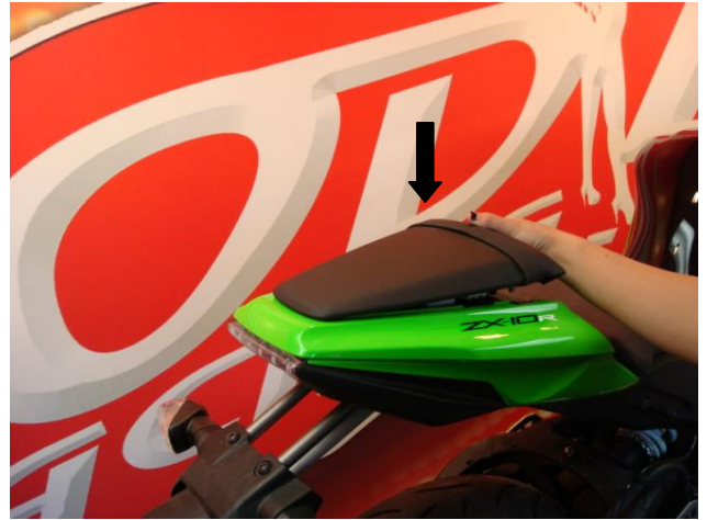
36. Install passenger seat.
