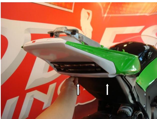
27. Insert pop rivets into bottom of the undertail.
