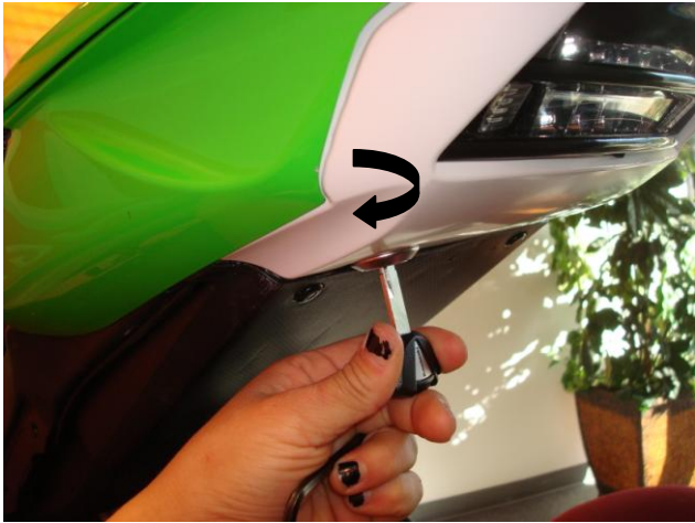
35. Ensure proper passenger seat release.
