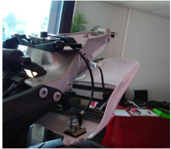
24. Attach the cable to the lock mechanism.
