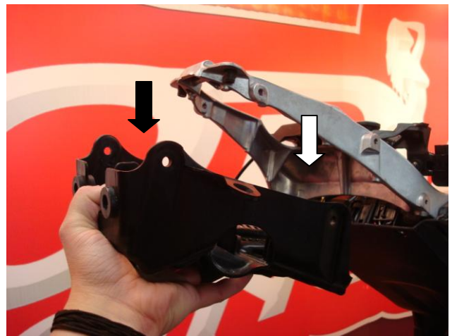
14. Remove the stock storage compartment.
