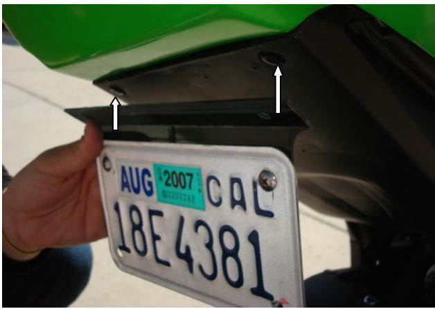
31. Use supplied bolts to mount license plate. (Position depends upon personal choice)
