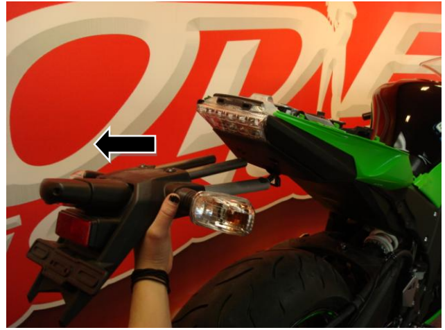
6. Pull mud flap to remove.
